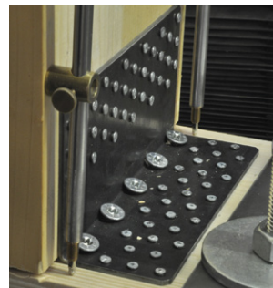
Tension test: full nailing
