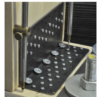
Tension test: partial nailing
