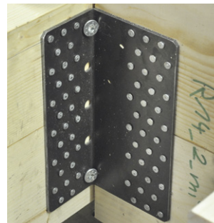
Shear test: full nailing
