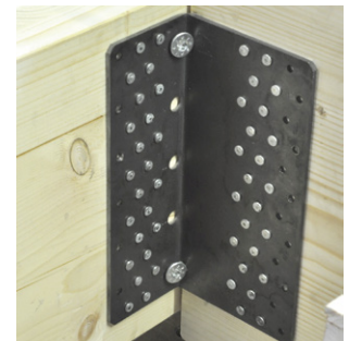
Shear test: partial nailing
