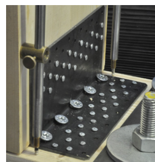
Tension test: partial nailing
