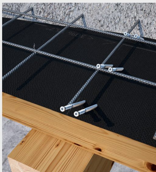
Composite timber-concrete floors with 30° connectors arranged in a double row.
