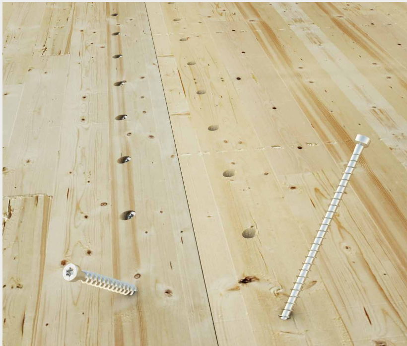
Very high stiffness in side-by-side joining of CLT floors. Application with double inclination at 45°, the JIG VGZ template.
