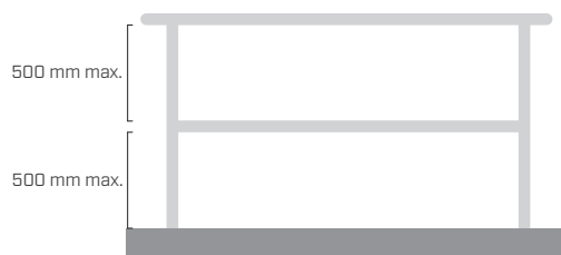
RAILING WITHOUT TOE BOARD
