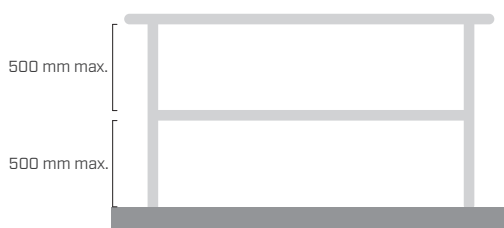
RAILING WITHOUT TOE BOARD
