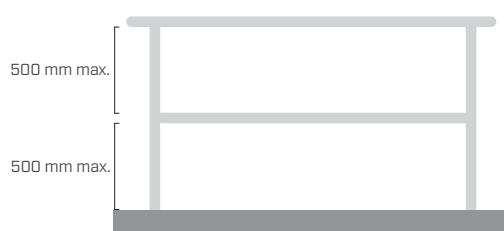
RAILING WITHOUT TOE BOARD
