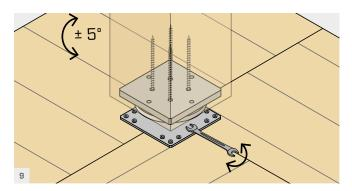
The slotted holes in the hexagonal disc allow the column to be rotated  $\pm 5^{\circ}$ . Turn the column to the correct position and tighten the 4 SPBOLT1235 bolts or hex nuts of the SPRODS, using a side wrench.
