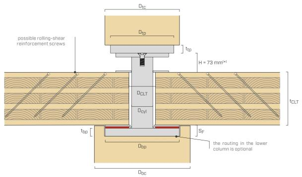
$<sup>^{(\</sup>star)}$  In case of application without XYLOFON WASHER and distribution plate (H = 85 mm). In case of application of XYLOFON alone (H = 79 mm).
