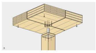
Fit the pre-drilled CLT panels with a circular hole of  $D_{\text{CLT}}$  diameter onto the cylinder. A compression reinforcement can be provided to the panel bottom of beam to increase strength.
