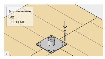
Connect the FASTENING PLATE to the CLT panels with 12 HBS PLATE 8x120 screws.
