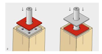
Insert the XYLOFON WASHER (optional) and/or the DISTRIBUTION PLATE (optional) on the cylinder.
