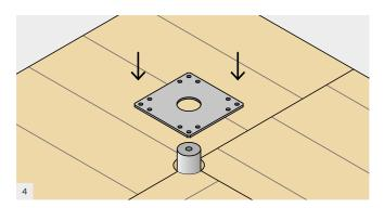
Insert the FASTENING PLATE onto the cylinder.
