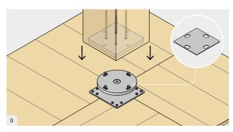
Place the upper column on the disc and fasten it using 4 SPBOLT1235 bolts with ULS125 washer. In the case of upper steel column, the upper plate must not be used and the column must be equipped with a suitable steel plate with holes for fastening the 4 SPBOLT1235 bolts.
