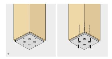
Fasten the upper plate to the lower face of the column using the VGS  $\emptyset$ 11 screws, in accordance with the relevant installation instructions. The top plate is equipped with suitable threaded holes for fastening to the disc. If SPRODS are used, after positioning the plate on the upper column, they must be screwed in, taking care to mark the minimum pull-through length in the upper plate.
