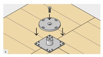
Place the DISC on the CYLINDER and fasten the countersunk head screw with a 10 or 12 mm male hexagonal wrench.
