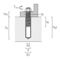
internal threaded rod diameter ď diameter of the element anchored on concrete  $\mathsf{d}_0$ hole diameter in the concrete support  $h_{\text{ef}} \\$ effective anchoring depth  $d_{\mathsf{f}}$ hole diameter in the element to be fastened T<sub>inst</sub> maximum tightening torque  $\mathsf{t}_{\mathsf{fix}}$ maximum fastening thickness  $h_1$ minimum hole depth length of internal threaded rod
