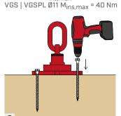
Length and quantity of screws depend on the application and the weight of the element to be moved. It is recommended to tighten them in accordance with the tightening torques indicated in the relevant installation instructions.
