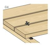
It is recommended to use STAR spacers inserted between the boards.
