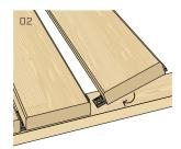
Turn the board over and slide it under the previously fastened board fixed to the sub-structure.
