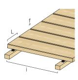
i = i = joist spacing L = board width | <math>f = joint width
