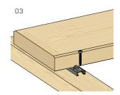
Fix each fastener to the sub-structure by inserting a KKTX screw in one of the two slotted holes.
