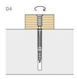
Attach the batten, screwing in the screw so that the head is flush with the timber.
