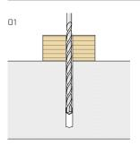
Drill the elements with a  $d_V$ = 0.20 inch diameter.
