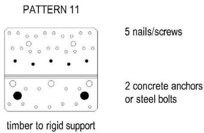
Figure B. 14 Nailing patterns for Angle Bracket NINO 15080
