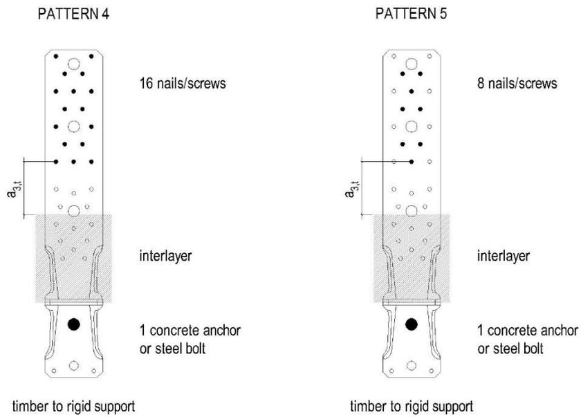
Figure B. 35 Nailing patterns for WKR285
