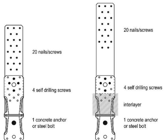
Figure B. 38 Nailing patterns for WKRD40 and WKRD60
