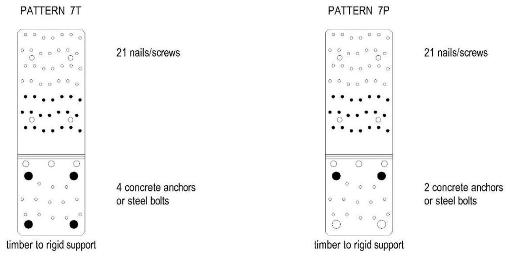
Figure B. 18 Nailing pattern for Angle Bracket NINO 100200
