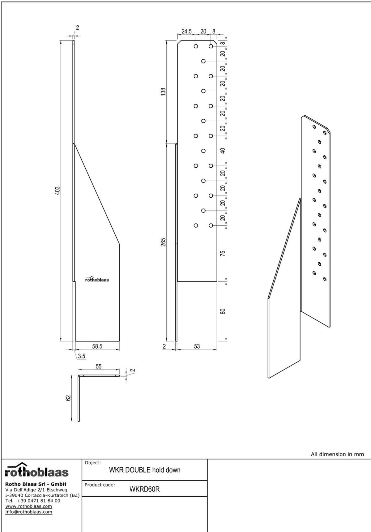
Figure B. 28 Dimensions of Rotho Blaas WKRD60R
