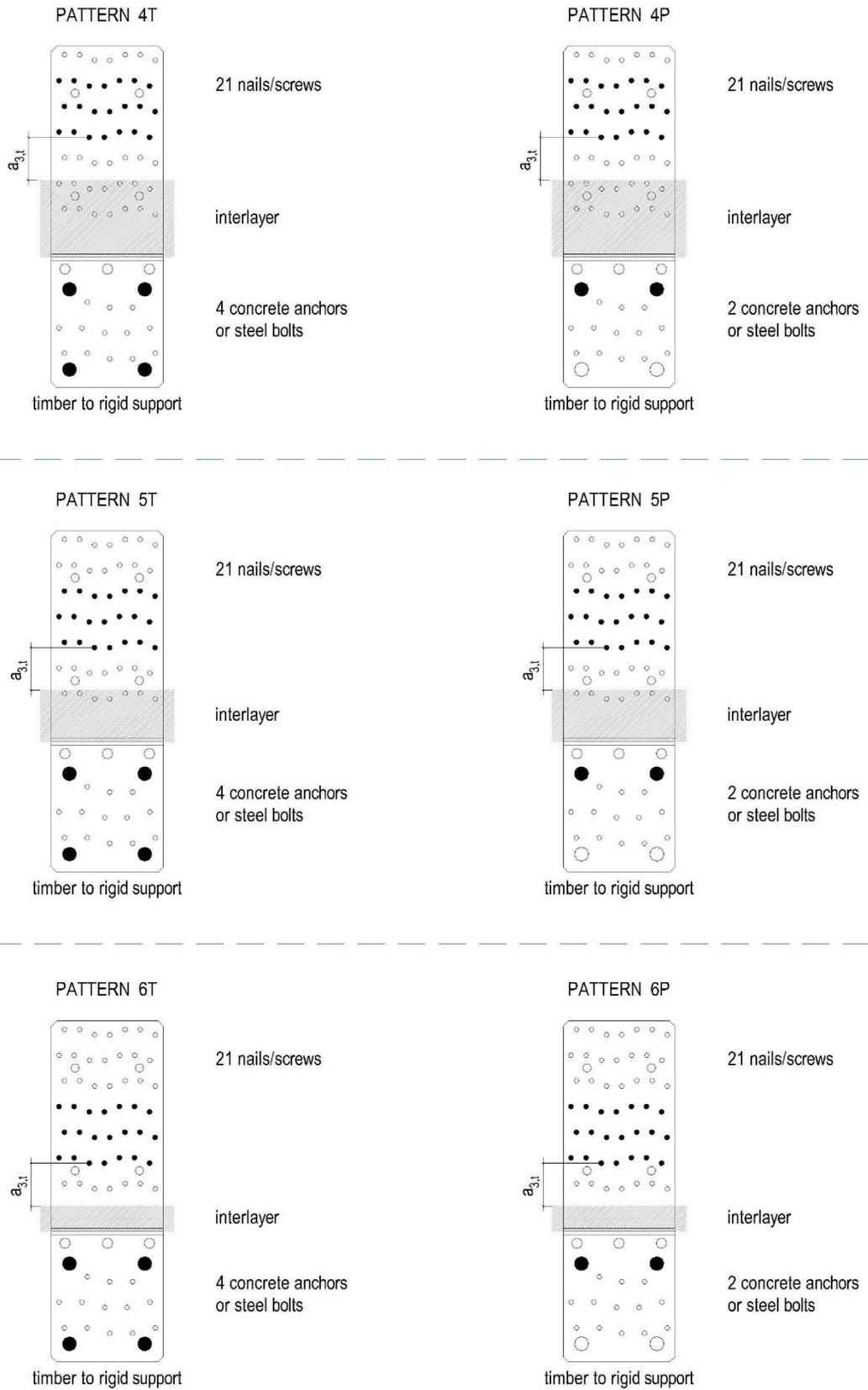
Figure B. 17 Nailing patterns for Angle Bracket NINO 100200
