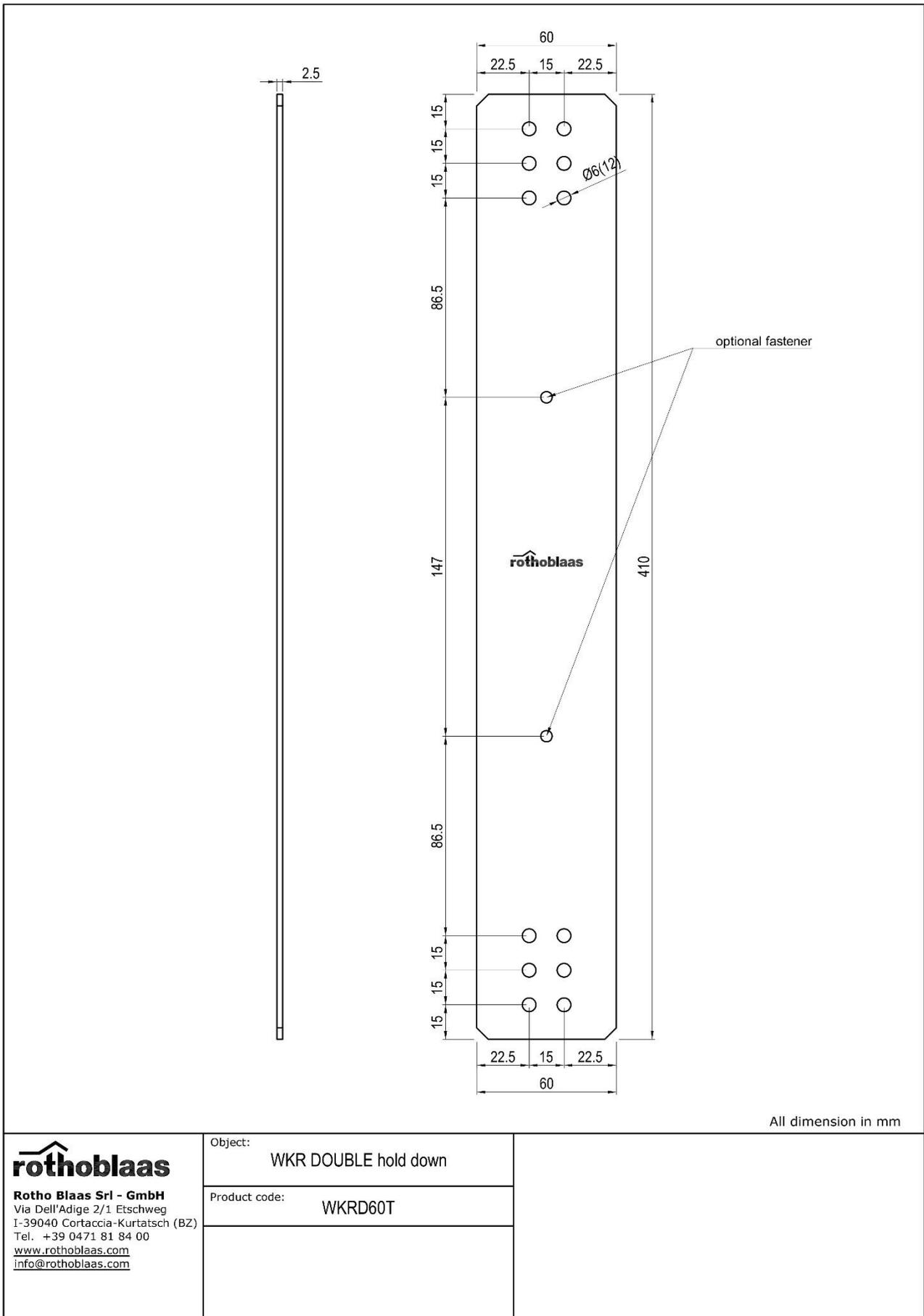
Figure B. 29 Dimensions of Rotho Blaas WKRD60T
