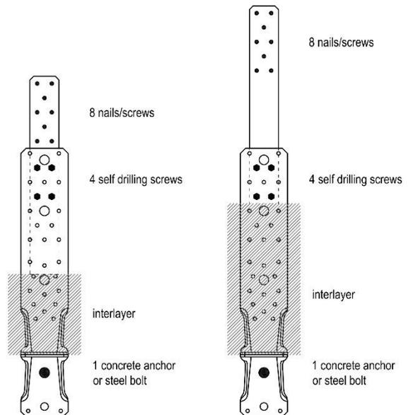
Figure B. 37 Nailing patterns for WKR410 and WKR 530
