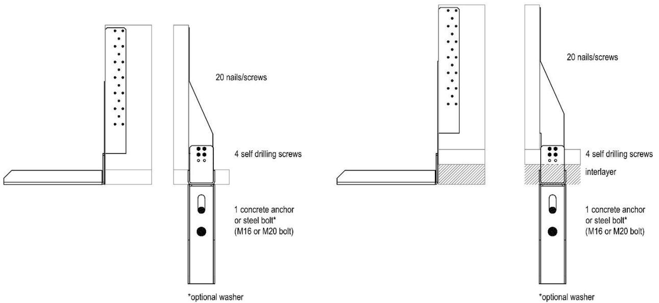
Figure B. 41 Nailing patterns for WKRD60L, WKRD60R and WKRD100C
