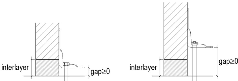
**Table B.14:** Force  $F_1$ , head pull-through capacity of a fastener in the horizontal flange
