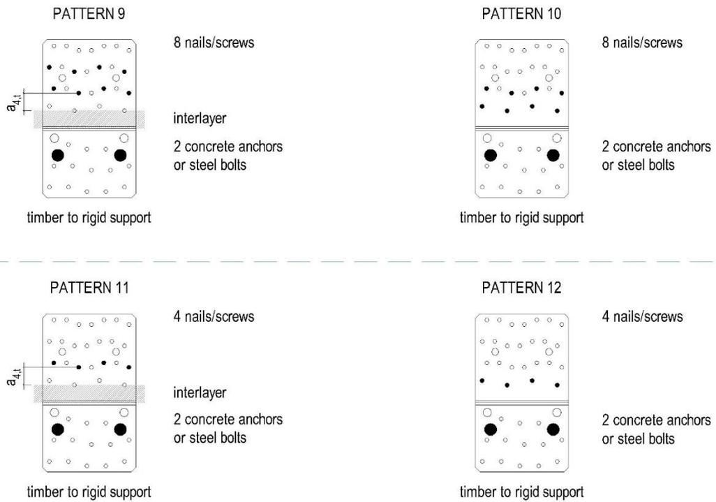
Figure B. 12 Nailing patterns for Angle Bracket NINO 100100
