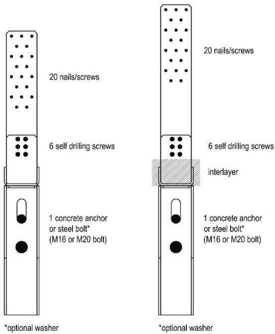
Figure B. 39 Nailing patterns for WKRD60 and WKRD100C
