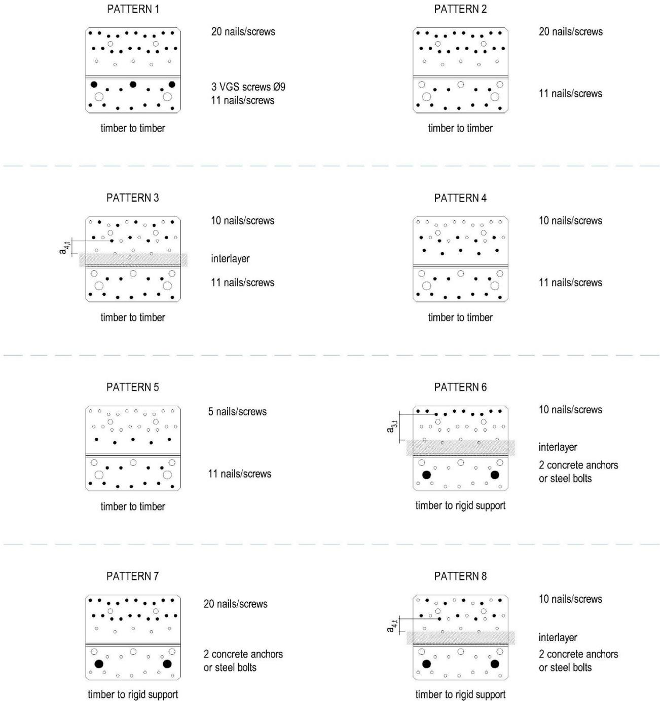
Figure B. 13 Nailing patterns for Angle Bracket NINO 15080
