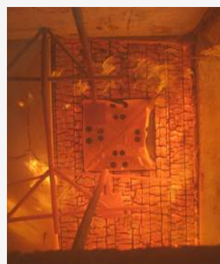
Fire performance of the X-RAD system in the test chamber (sample A not coated)
