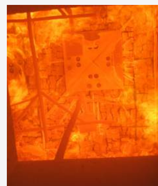
Fire performance of the X-RAD system in the test chamber (sample A not coated)
