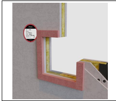
Figure B.1: Opening frame in flexible walls.
