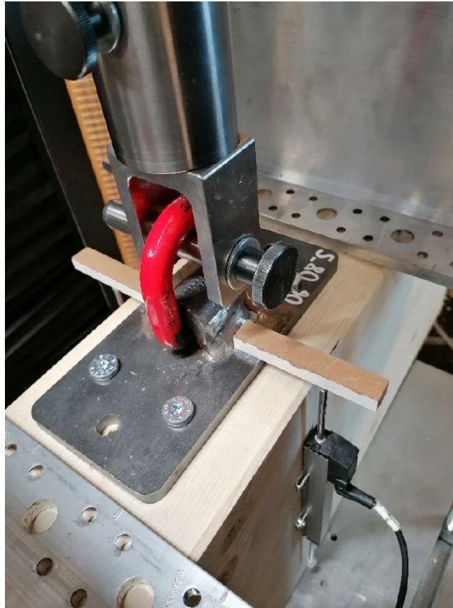
Figure 8. Photo of the test rig used for the repeated-use screw-level tests at Rothoblaas.
