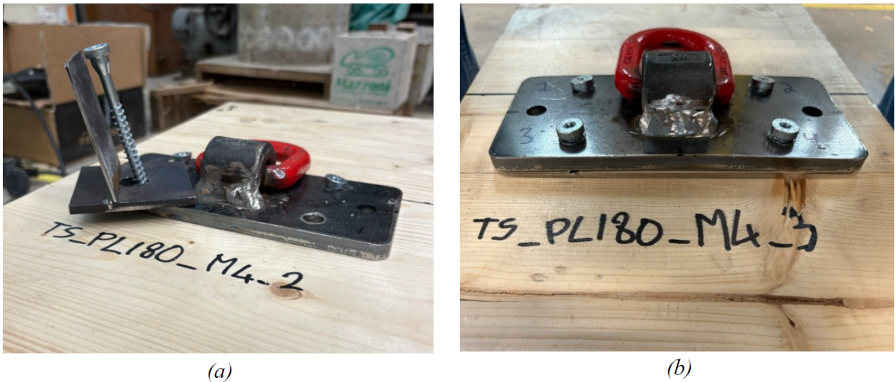
Figure 25. (a) Insertion of the screw at an inclination of 10^\circ using a dedicated jig; (b) Screws in place after installation, inclined at 10^\circ (MECH 4).
