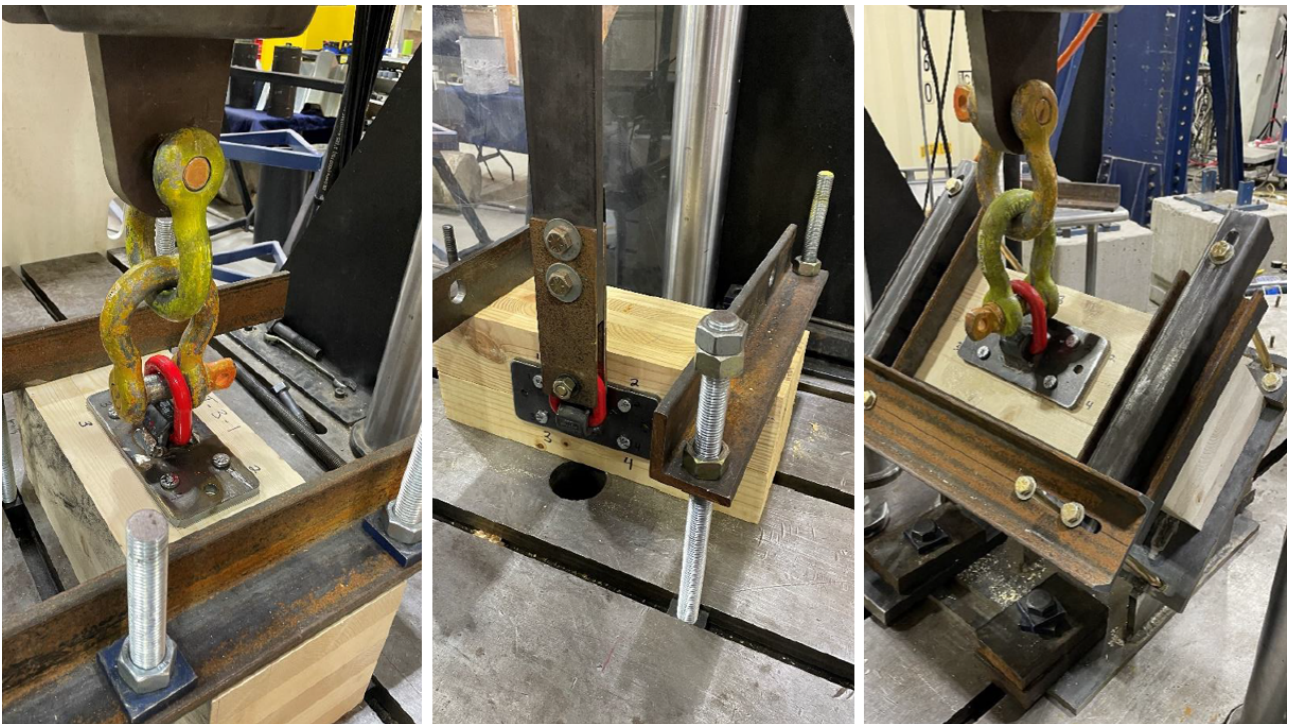
Figure 14. Test setups for pure tension (load applied at 90° to the panel surface), pure shear (load applied at 0° to the panel surface), and combined tension-shear (load applied at 45° to the panel surface).
