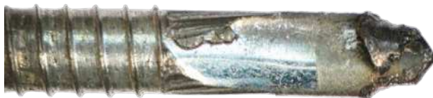
Tip melted during installation on a too hard plate without spacers between timber and plate.
