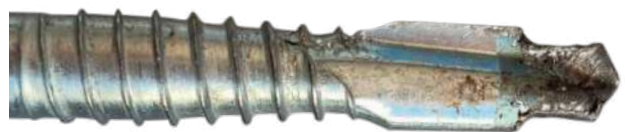
Reduction of the tip when drilling the plate due to the high hardness of the plate.
