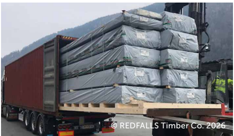
Additional protection of the panels in the case of long journeys or possible exposure to corrosive agents.
