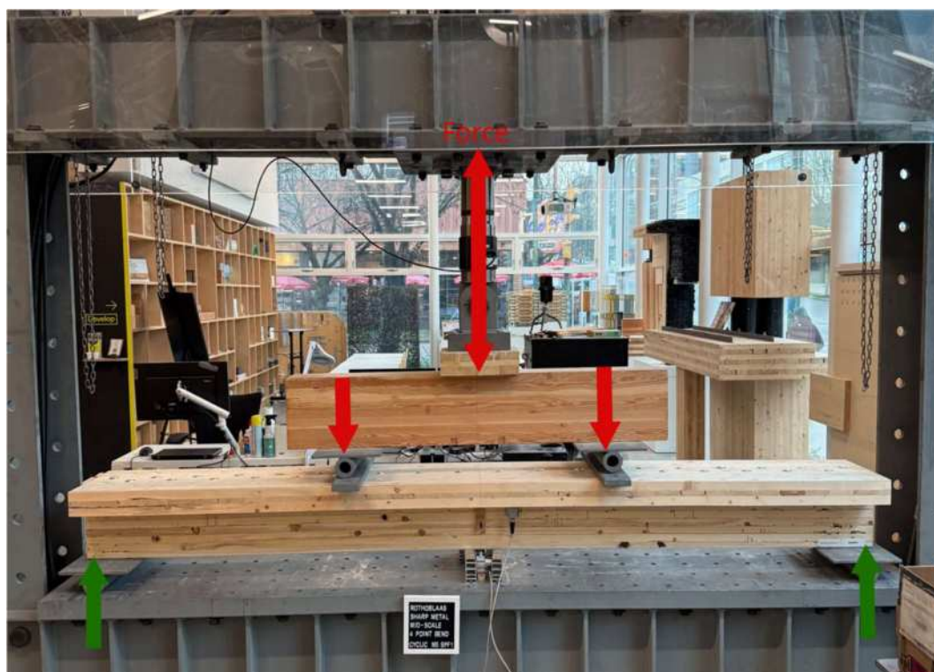
Picture 4: Mid-scale test specimens-load distribution and test setup.
