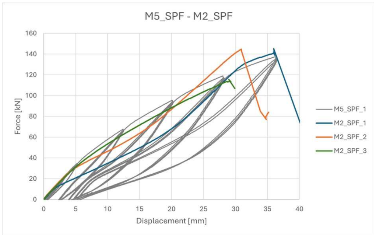
Picture 47: Cyclic test M5_1 (screws + SHARP METAL)- and monotonic tests M2 SPF timber.
