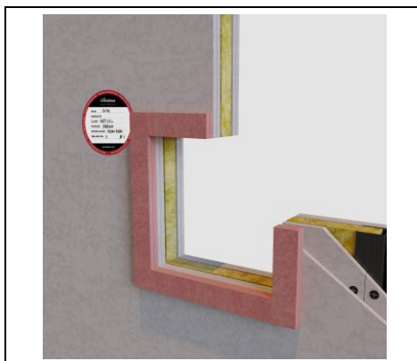
Figure B.1: Opening frame in flexible walls.
