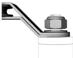
Correct installation of PATROLANG on TOWER - TOWER22 - TOWERA2 support
