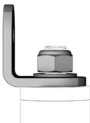
Installation correcte PATROTERM sur le support TOWER - TOWER22 - TOWERA2
