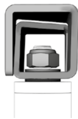
Installation correcte PATROLINT sur le support TOWER - TOWER22 - TOWERA2
