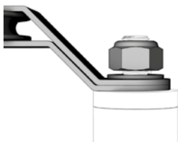
Correct installation of PATROLANG on TOWER - TOWER22 - TOWERA2 support
