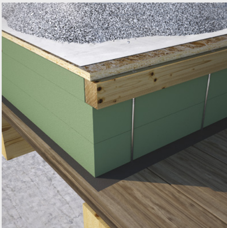
^ Fastening of hard insulation on a flat roof.
