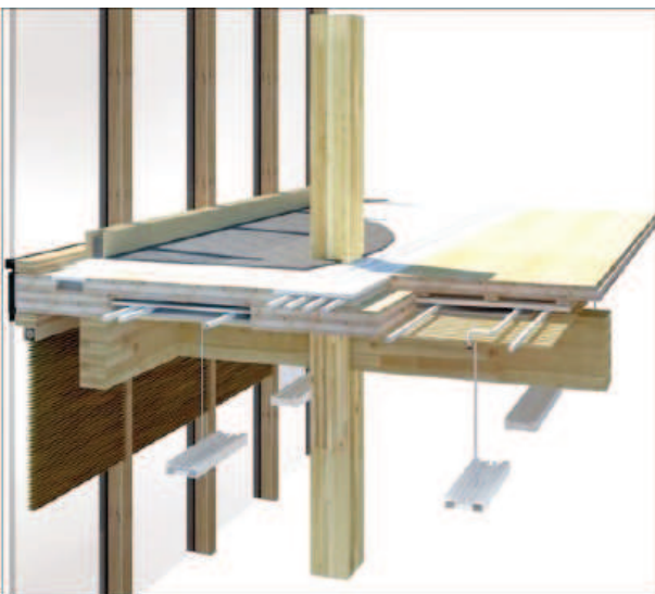
UBC – Wood Innovation Design Centre - Column-Beam system,
