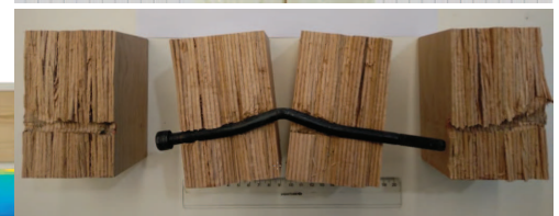
Steel yielding, Grade 12.9, f_y = 1400 MPa, numerical model for connections
