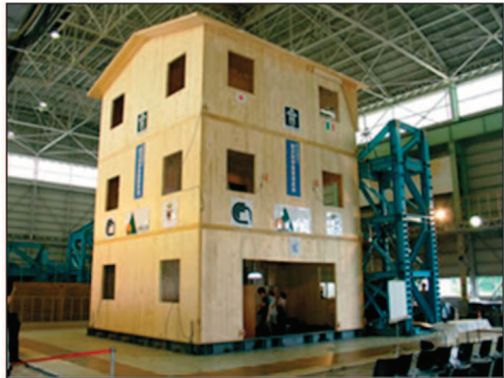
Fig. 5: Three-storey test building on the shaking table at NIED Laboratory in Tsukuba, Japan (configuration C)
