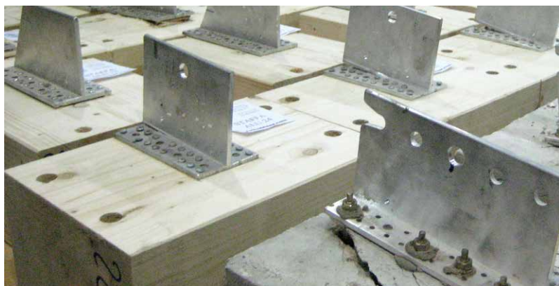
Tests on specimens with reduced dimensions (timber-to-timber and timber-to-concrete).
