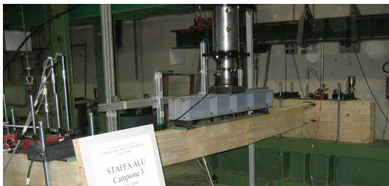
Tests on full-scale specimens (main-secondary beam connection).
