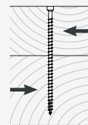
Angle between strength and grain \alpha = 90^\circ
