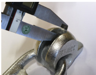
Method to measure minimum shank thickness m_{min}
