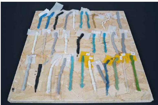
Test campaign to evaluate the adhesion, cohesion and elasticity of different glues and sealants.
