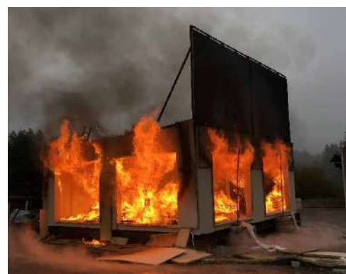
D. Brandon, J. Sjöström, A. Temple, E. Hallberg, F. Kahl, "Fire Safe implementation of visible mass timber in tall buildings - compartment fire testing", RISE Report 2021:40
