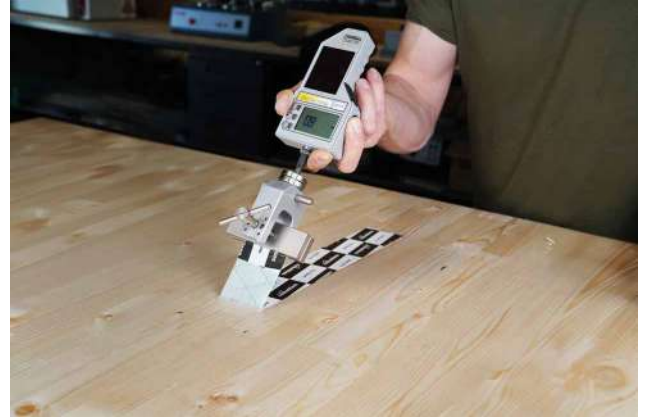
Test campaign on the cohesion and adhesion performance of acrylic adhesive tapes on different substrates.
