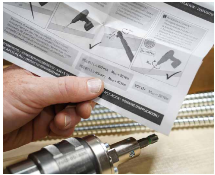
Accurately check the torque limit value specified for the screw.
