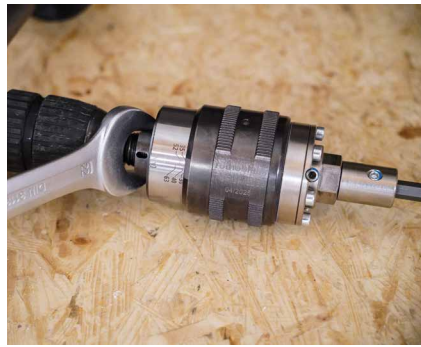
Set the TORQUE LIMITER to the correct torque value.
