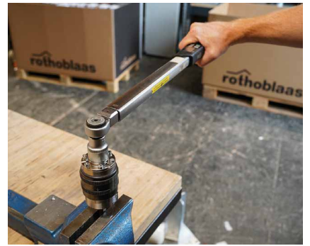
Perform an initial torque check with a torque wrench.
