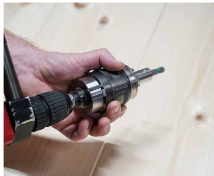
Turn the outer sleeve to reset the TORQUE LIMITER.
